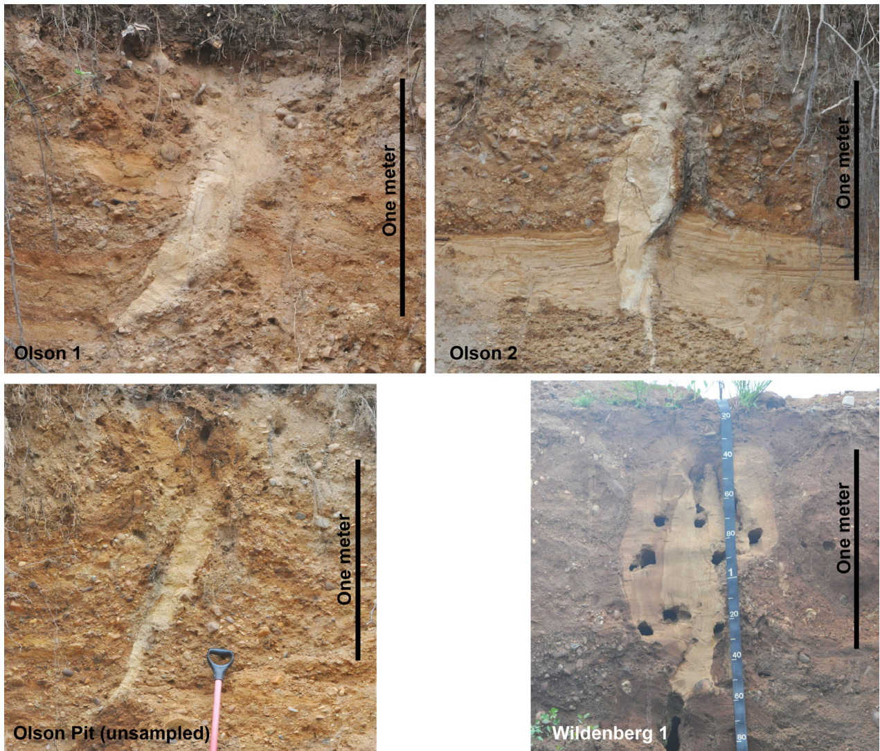
Fig. 11. Examples of upturned strata at the margins of sand wedges at the study sites.
